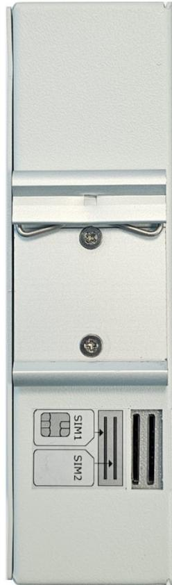
Note that the SIM1 and SIM2 cards are inserted in reversed direction.
